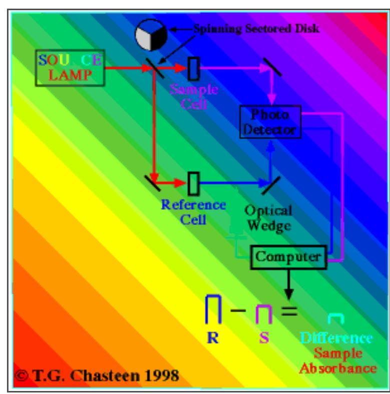
The alternating light signals, from either the reference beam or sample beam generate alternating electrical phototransducer signals. A computer, sampling those
