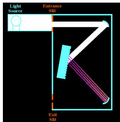
Since light passes off the grating at angles dependent upon its wavelength, it will also reflect off the mirror “down stream” at different angles. The further away from the dispersion element—and here’s the important part—the further apart will be the colors of light (read wavelengths) in the dispersing beam.
