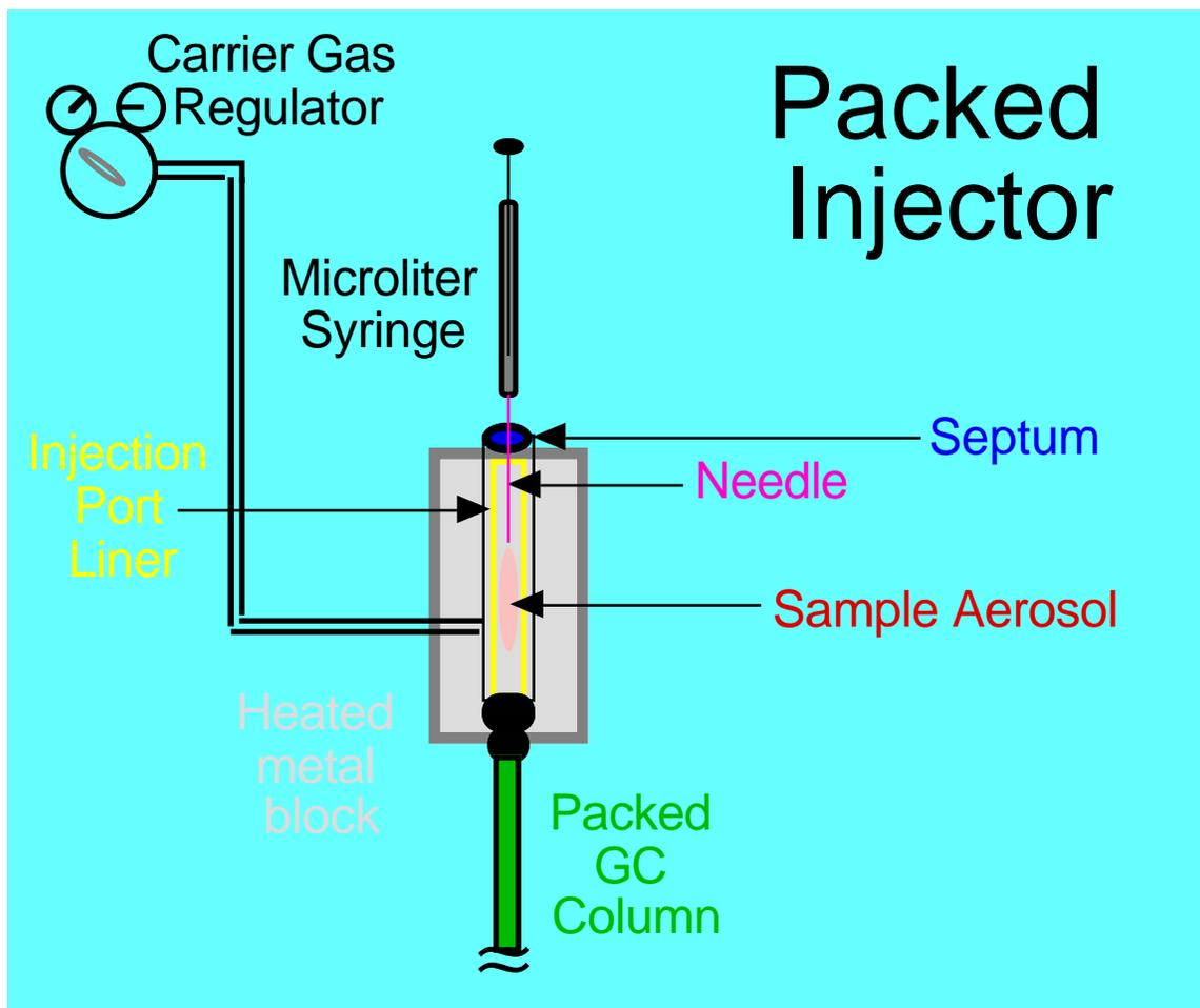
One last subtle point about the configuration of the carrier gas inlet: notice that it enters the injector at about the middle of the heating block and its gas has to travel along the outside of the injector before it enters the injection port liner AT THE TOP. This is so the carrier is preheated before it enters the liner where the sample is vaporized. This helps to prevent a cold spot at the top of the injector where the carrier gas enters.
