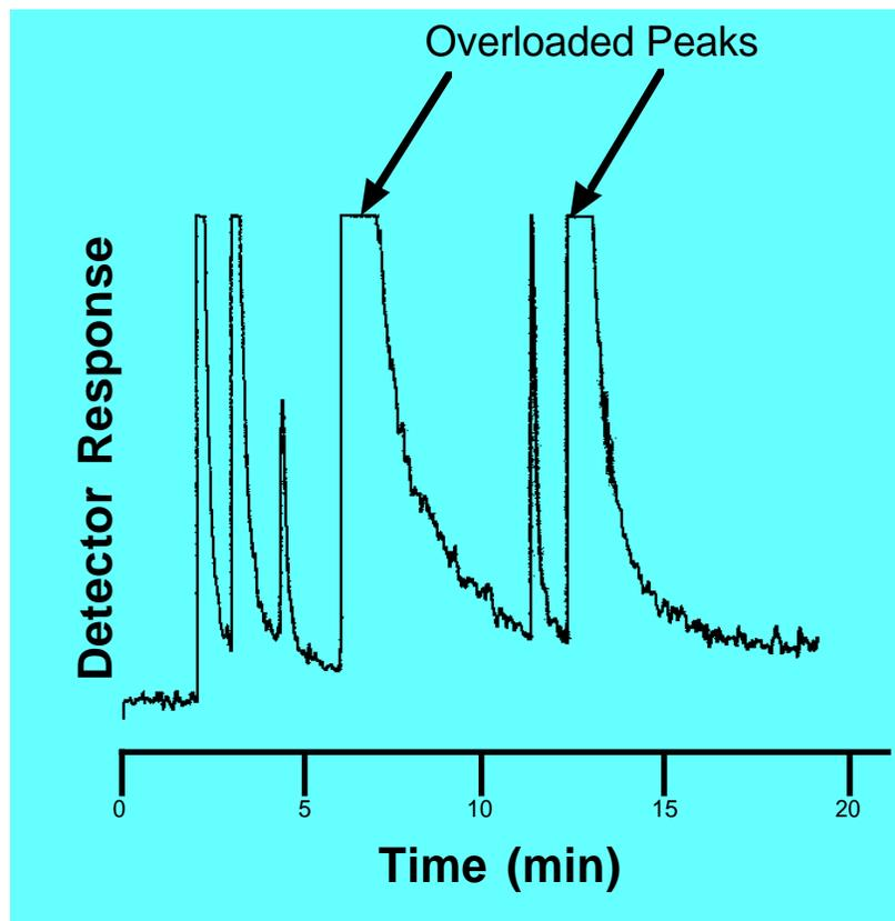
The following figure shows a little better chromatography with fewer overloaded peaks. The second eluting peak (about 6 minutes) is clearly not overloaded while the group between 10 and 14 minutes still shows overloading characteristics: long drawn-out tailing and much less than baseline separation with peaks that elute nearby (the 11 and 12 minute peaks, for instance).
