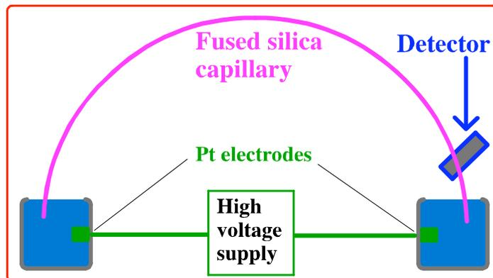
Because of the small diameter of the typical CE capillary (25 to 100  $\mu\text{m}$ ), CE sample volumes are some of the smallest of any modern separation method. Sample volumes for HPLC are routinely 20  $\mu\text{L}$ ; those of capillary GC, 0.5 to 1  $\mu\text{L}$ . But CE sample volumes are 50, 10, even 1 nanoliter (nL) or less. 1 nL!
