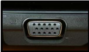
Your monitor or projector will come with a VGA cord that will connect the two devices. Once you have the two devices connected, power on your laptop and your monitor or projector. If you are having trouble with the display you may have to press the key combination of Function key (Fn) which is located between the CTRL and ALT key + F4 key to get it set up correctly. It may take pressing that key combination (Fn + F4) more than once to toggle between the different settings.
