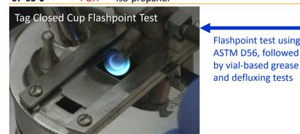
Promising azeotropes were prepared for use in the vapor degreaser in performance tests in comparison to TCE and nPB.
