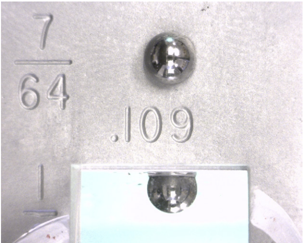
FIGURE 5.12 A nominal 119° SRO constructed using a 3.18 mm chromium steel ball in a 2.77 mm drilled gauge hole viewed from above and from the side using a prism.
