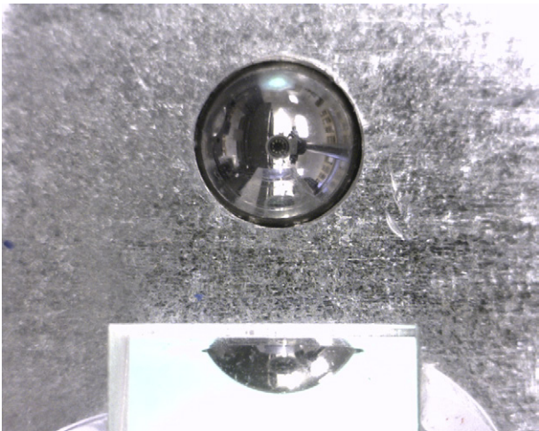
FIGURE 5.13 A nominal 54.3° SRO constructed using a 6.35 mm chromium steel ball in a 5.16 mm hole drilled in galvanized metal sheeting viewed from above and from the side using a prism.
