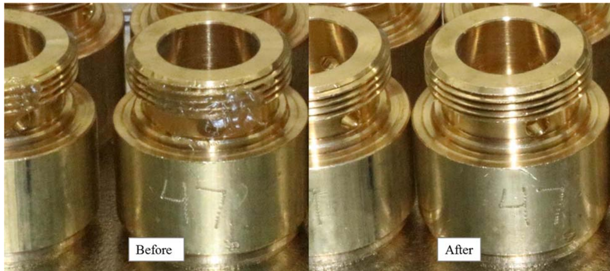
Figure 23: The visual performance of nPB in the Branson 125 against marine grade grease on brass fitting #47 shows that the degreasing protocol works well. The visual performance of TCE was identical.
