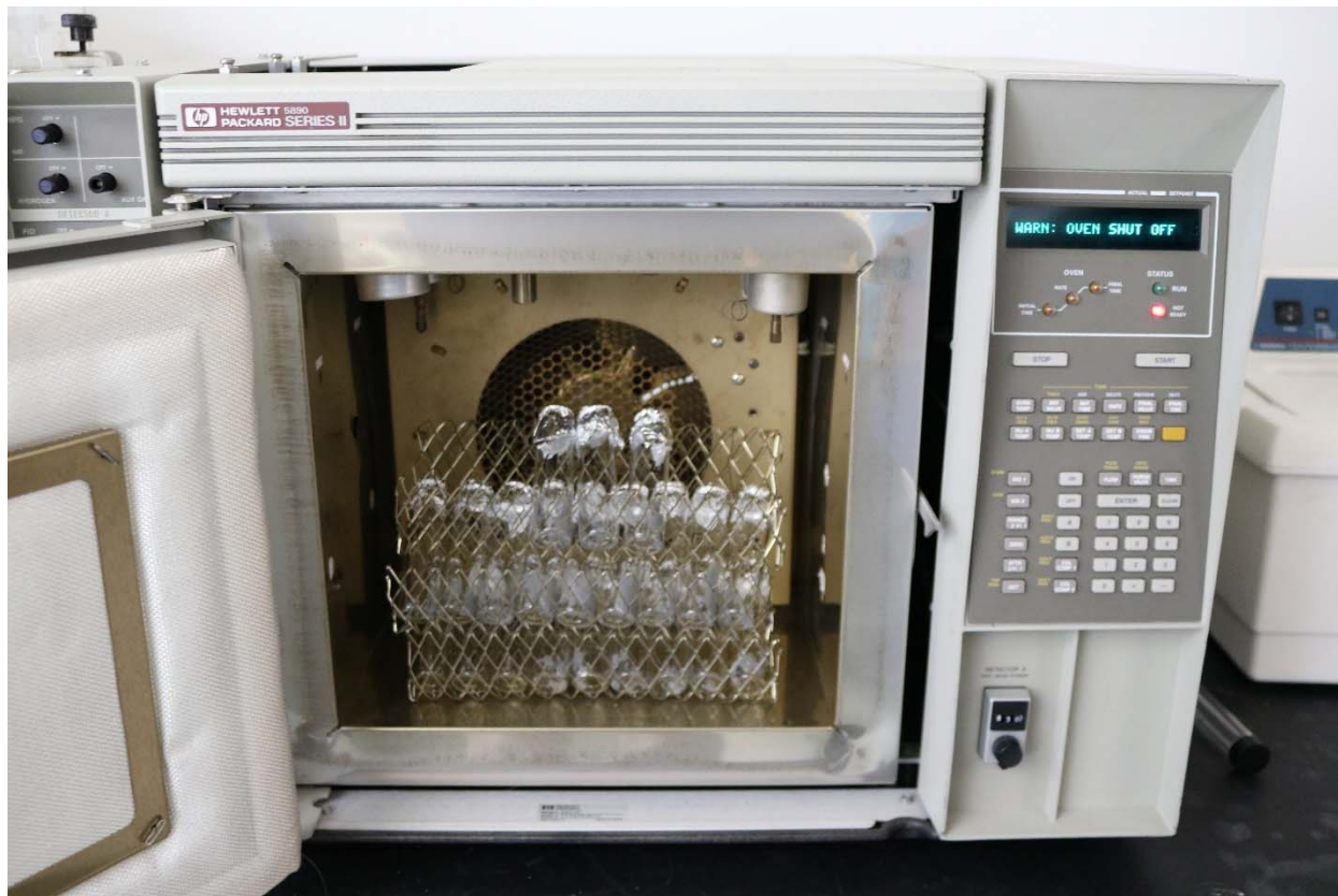
Figure 8: The HP 5890 GC oven that served as a temperature-programmable reflow oven for the vial-based defluxing tests
