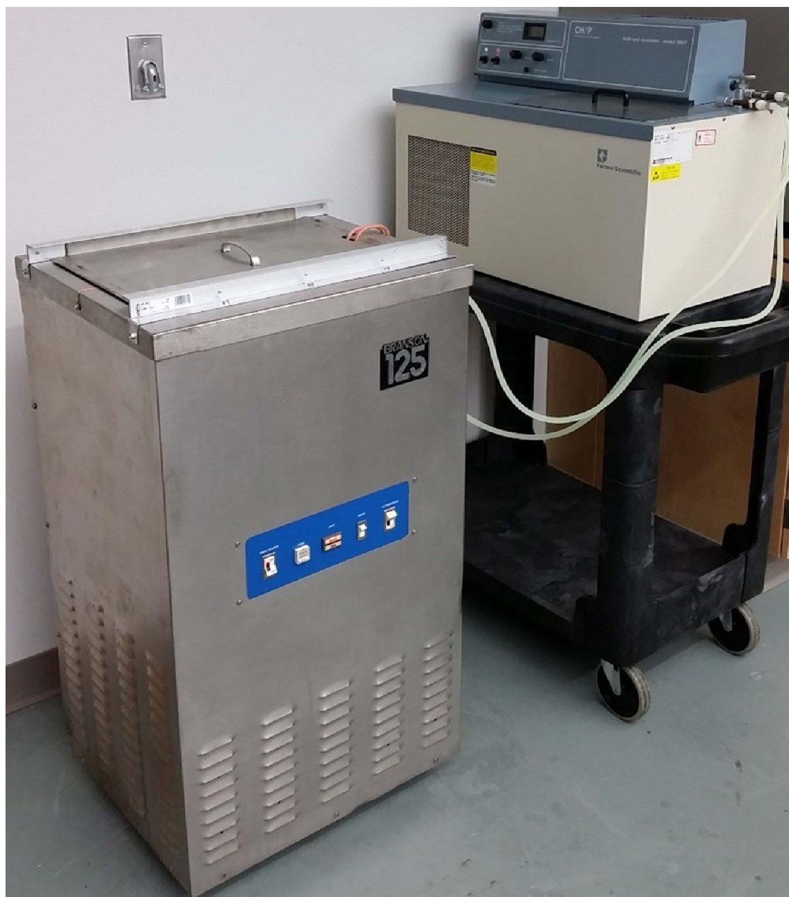
Figure 4: The 7.6-L (2-gallon) capacity Branson 125 vapor degreaser retrofitted with a sliding lid and sub-zero coils
