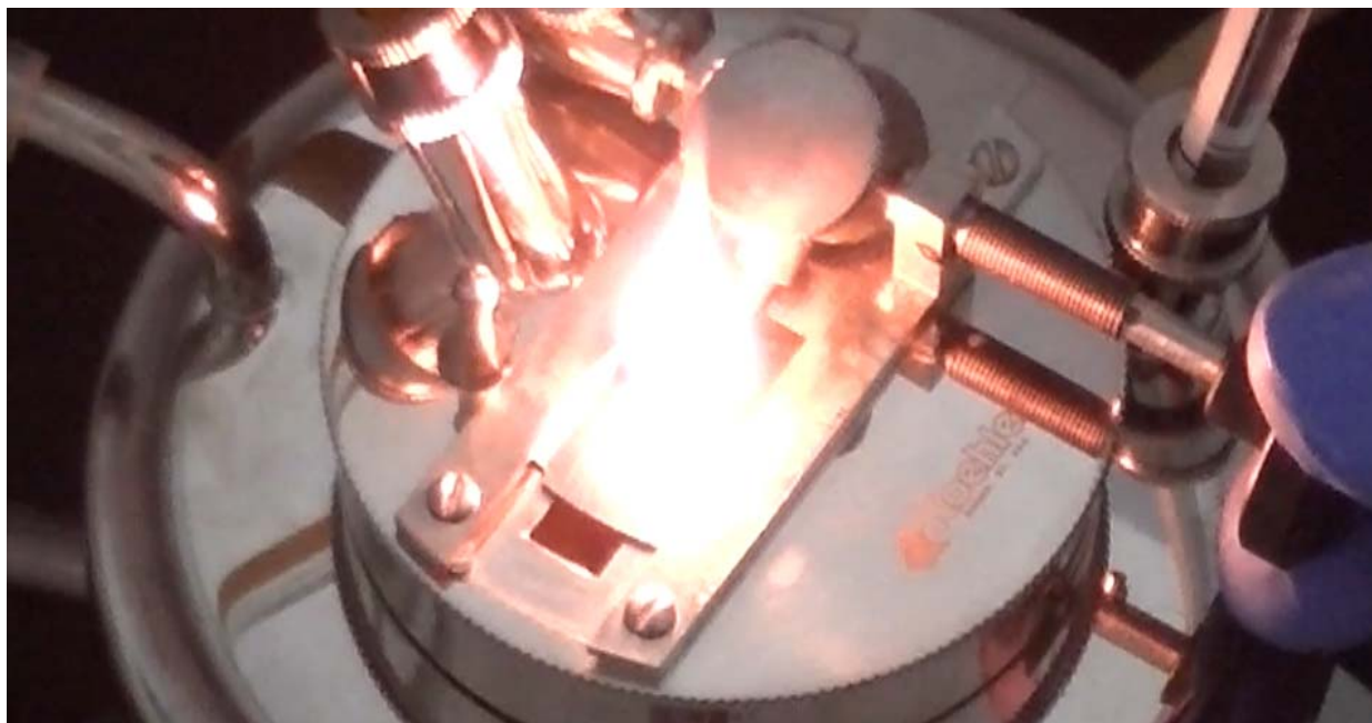
Figure 19: Photo of HFE-7100 participating in burning up to its boiling point
