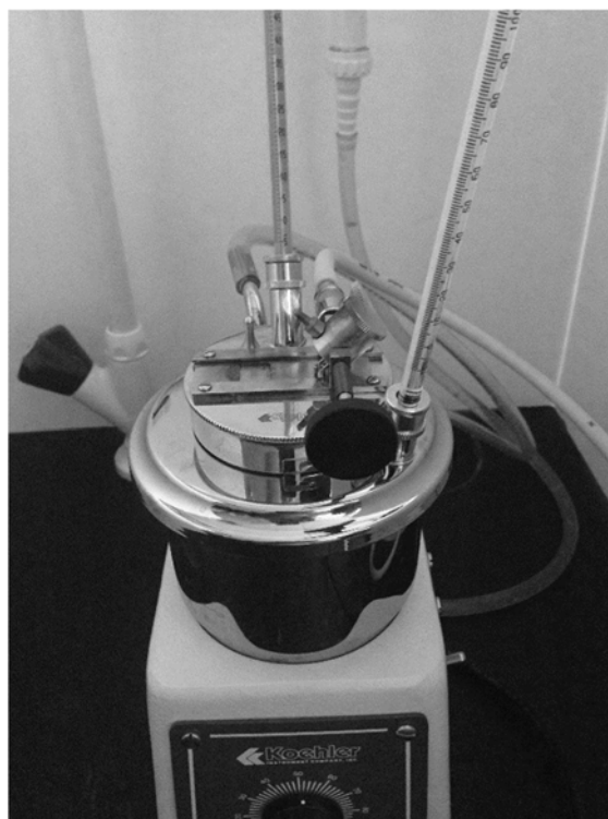
Figure 10. Koehler Model K14600 tag closed-cup flash point apparatus.
