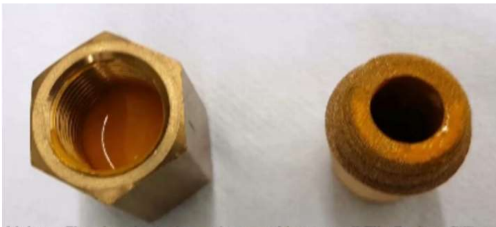
left side: capping nut, bottom closed and filled with riboflavin right side: open-pored filter (pore size 70-90 microns), screwed in the nut
