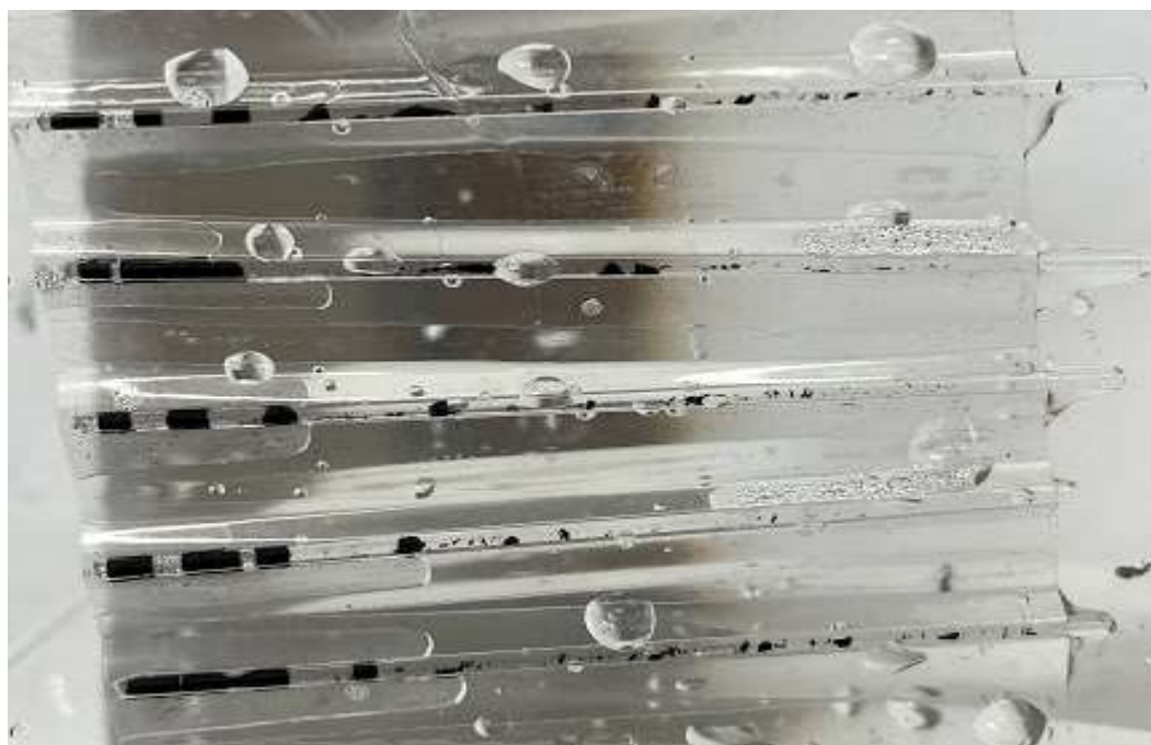
Figure 21. Effect of ultrasonic vibration in horizontal dry capillary tube cleaning.
