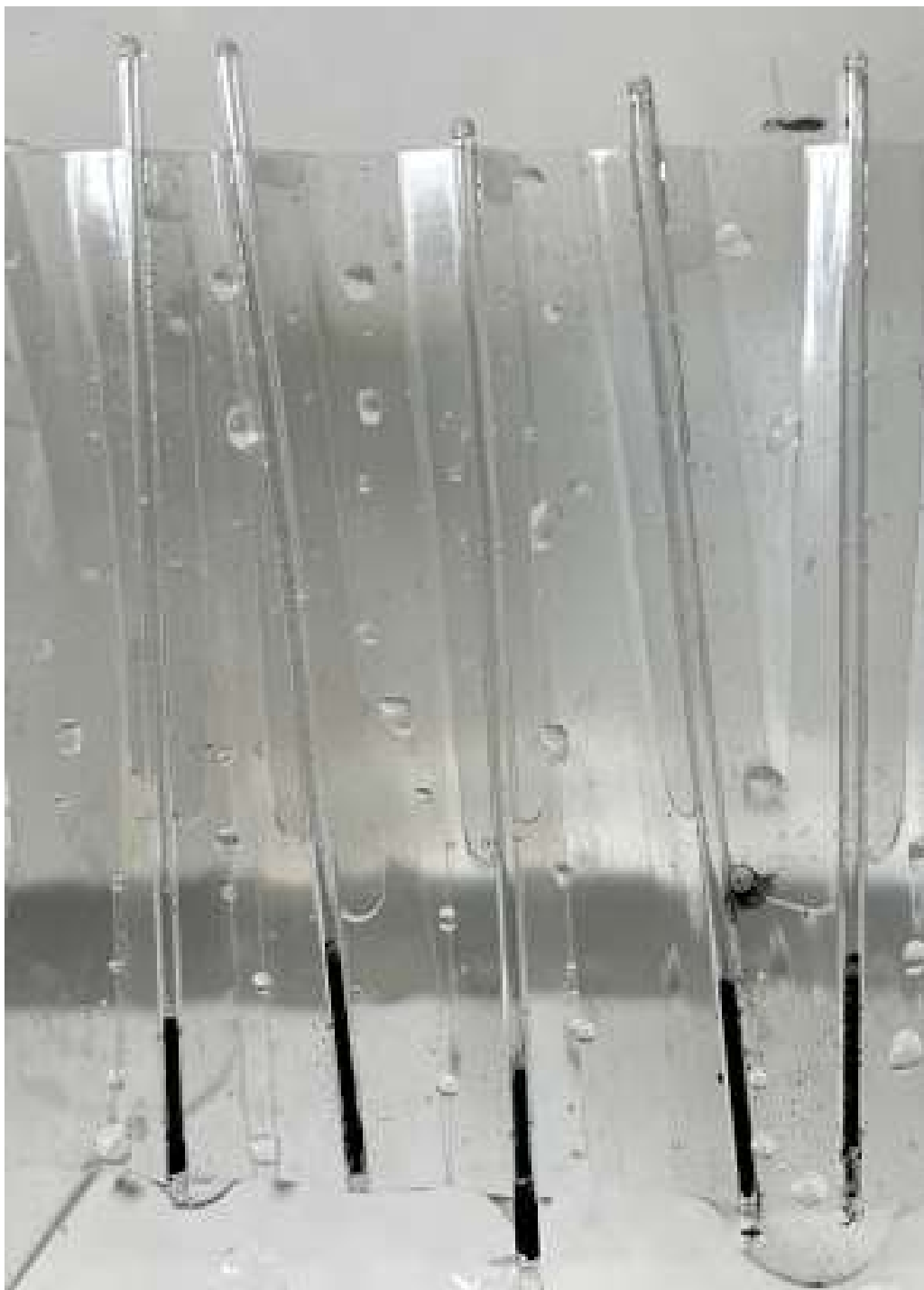
Figure 22. CB powder is stuck in the tip of the capillary tubes in vertical dry UC cleaning.
