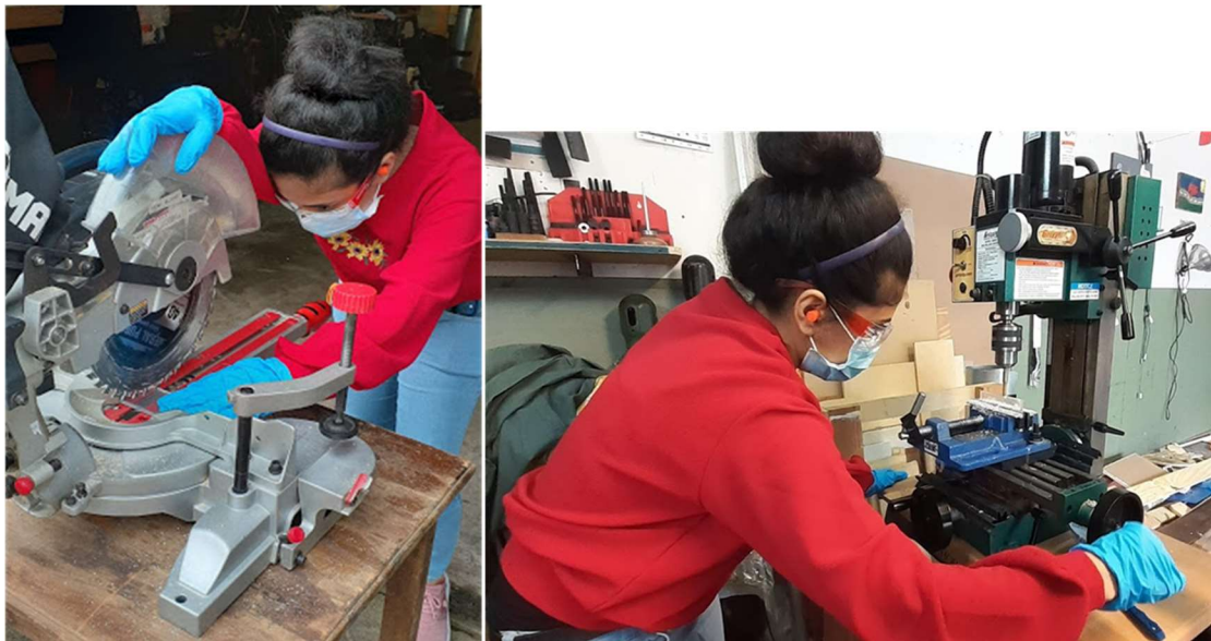
Figure 12. Making plexiglass windows using the miter saw (left) and mill (right).
