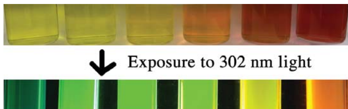
CdTe nanoparticles fluoresce when exposed to 302 nm UV light.
