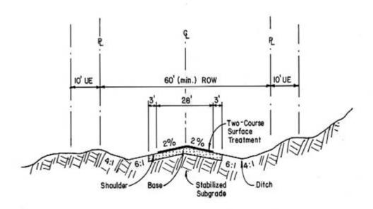
Surface material shall consist of two-course surface treatment comprising of P-3 and P-4 aggregate as (SDHPT) specifications item 304 at 35#/sy and 15#/sy, respectively and asphalt binder. Surface course shall be laid on prepared and primed flexible base. (SDHPT standard specifications for gravel, crushed rock; iron ore) placed on stabilized subgrade, both compacted to 95% Modified Proctor. Thickness of base depends on subgrade, material specifications and traffic characteristics.
